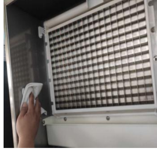
Scrub the inner wall of the ice sheet
